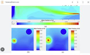
CFD simulation and experimental study of a hydrogen leak in a semi-closed space with the purpose of risk mitigation - ScienceDirect
