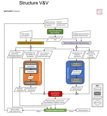
Fig. 1: A revised version of the MOTIVATE validation flowchart, updated relative to Hack et al.<sup>2</sup> following user feedback. The coloured boxes represent sub-charts broken out in tabular form over the next sections.
