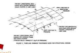
e.g. Design for Redundant Structures ...Tom Swift. For conventional metals, a cracked frame and 2 cracked frame bay skins
