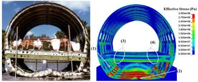
(a) Post-impact picture of section drop experiment
